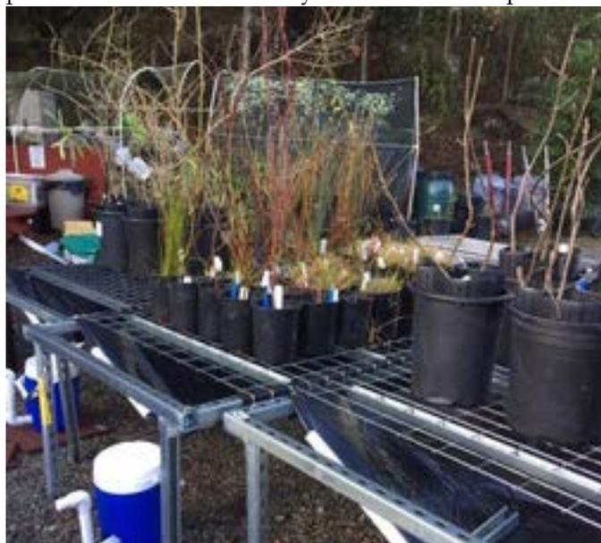
Left: Pear baiting test tables made by construction expert Per Brashears. Metal tables can be easily sanitized. Plants to be tested are placed on the tables, irrigated to create flow-through, and the water is collected in the vessels below. Unblemished pears are incubated in the effluent and inspected daily for characteristic phytophthora lesions.
